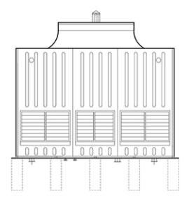
Flow rate based on temperature design condition at 100° F/37.7° C inlet and 90° F/32.2° C outlet with ambient WBT (Wet Bulb temperature) at 83° F/28.3° C.
