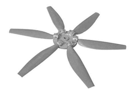
All FTA-4/6-F fan assemblies are dynamically balanced to provide zero vibration as well as corrected tip clearance and track variation. All fan assemblies are accompanied by a heavy duty cast aluminum/ss hub. All fan blades are adjustable in pitch, so as to completely utilize the rated horsepower.
